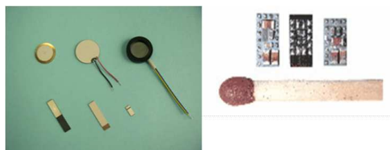
Figure 8. Piezoelectric converters, that are the basis of an ultrasound bone stimulator – ear noise masker (a), highly miniaturized signal processors used to generate dither noise at 30 kHz frequency (b)
